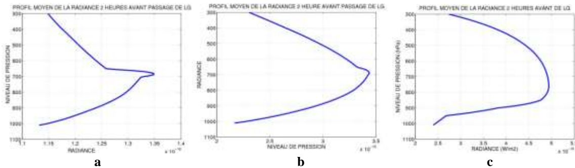
Figure 5. Average profile of Radiance 2 hours before the passage of squall line (SL) a) 50.31 GHz ; b) 53.73GHz ; c) 54.96 GHz
